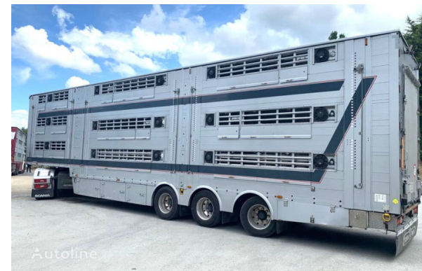
Figure 1 – A vehicle for transporting animals with a level system
