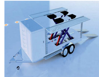
Figure 2 – Mobile Workshop in Conveyable and Working Positions
